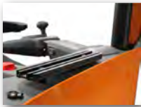
E-bar, with options to fit writing table, scanner, small item holder and PC
